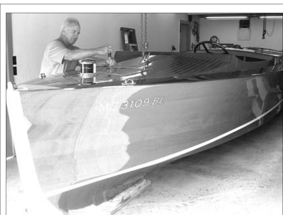
Master boat craftsman Jim Mertaugh of Hessel screws in newly chromed hardware around the hatch on the deck of Buddy.
