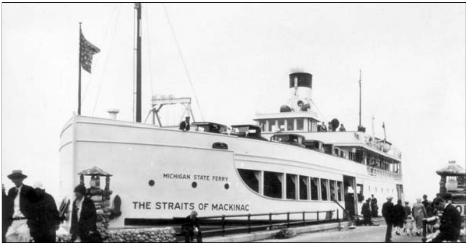
After sailing for only part of one season, The Straits of Mackinac was fitted with an upper cardeck capable of handling more than 20 additional automobiles. Her new capacity of over 80 cars was badly needed during the summer of 1929, before the stock market crashed. (Postcard, photographer unknown. Author's collection.)
