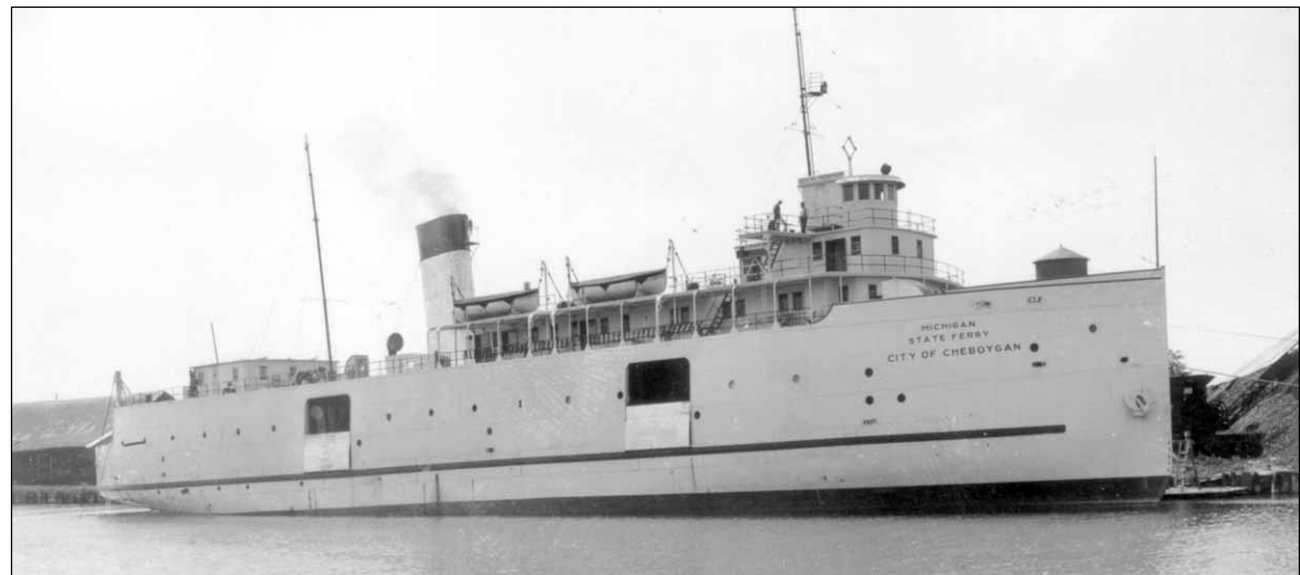
The City of Cheboygan conversion was done primarily at Lund's Shipyard on the Cheboygan River. Large side-loading openings were cut in the former Ann Arbor #4 's sides, the rails were removed from her cardeck, and, over the summer of 1937, she was made into the newest Michigan State Ferry. The work took longer than expected, and she wasn't ready for christening until August. (Postcard view, author's collection)
