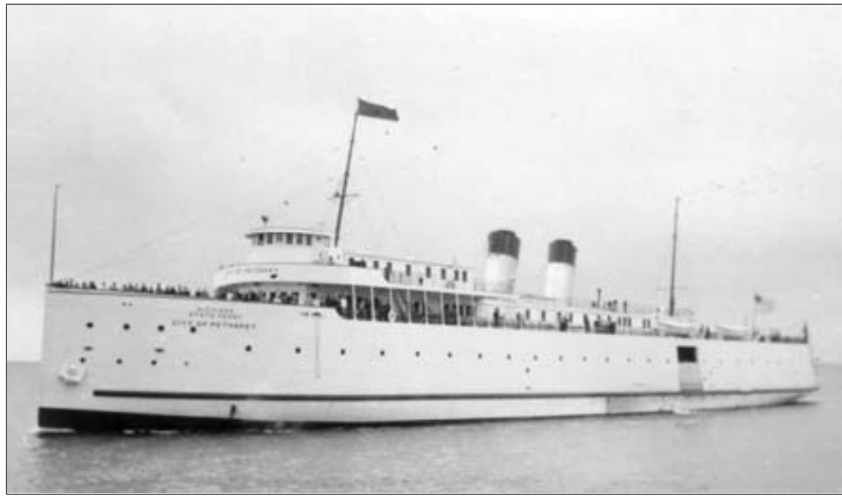
The City of Petoskey could most easily be distinguished from the similar looking City of Munising by her single side-loading ramp. The earlier-modified Munising had two, left over from the days when all the ferries loaded that way. By the time the Petoskey joined the fleet, end-loading ramps had been constructed. The Petoskey was also the first ship in the fleet to have sewerage treatment tanks onboard. The others just pumped raw wastes overboard. (Tourist's 1941 snapshot, author's collection)
