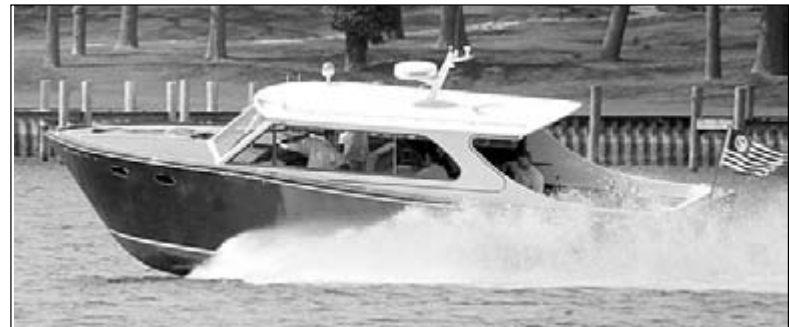
Grand Craft engineers and the Veneklasens test Music's twin Volvo, six cylinder diesel engines, which propel the boat up to 45 miles per hour.
