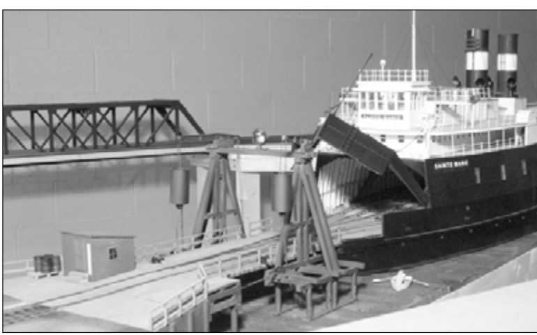
As seen in the photograph, the Sainte Marie's A-frame seagate would lift up to allow the captain, from the pilot house, to see to match tracks of the ship to those of the apron, which allowed the transport of railcars and automobiles to and from the ship. Steering the ship into port and lining up the tracks on the apron with the tracks on the ship was a tedious task.
