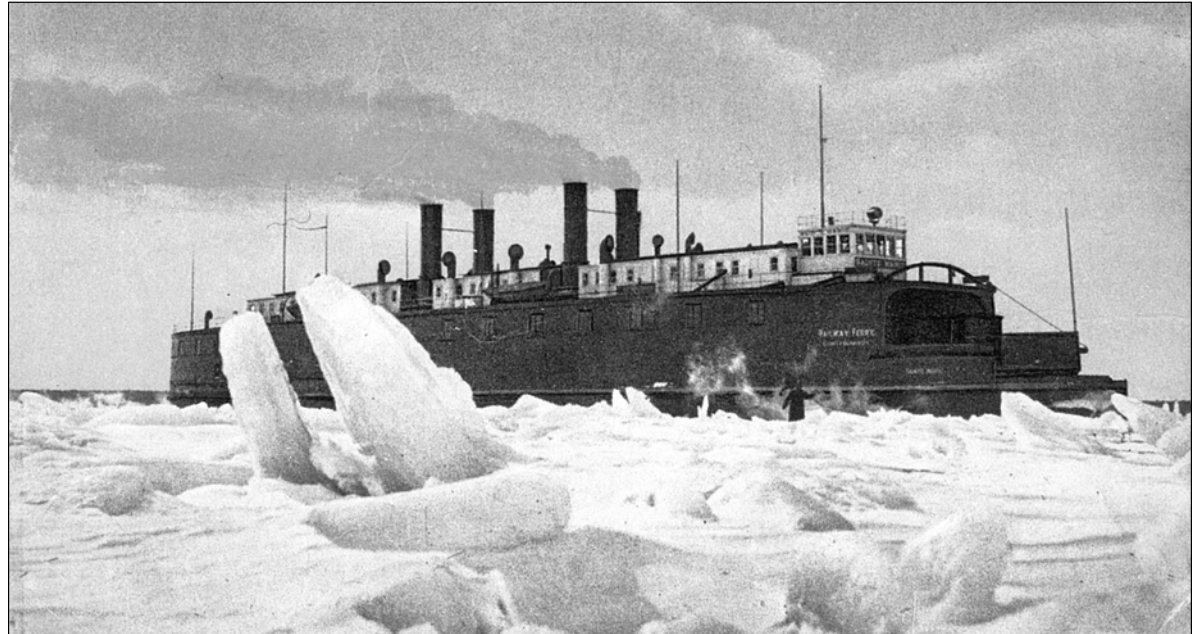
This postcard shows the 288-foot Sainte Marie , which ferried 18 rail cars across the Straits of Mackinac from 1893 until a newer rail ferry by the same name was put into service in 1913. The first Sainte Marie , which had a steel clad oak hull, had four stacks, while the later version, and the larger Chief Wawatam , had two. The original 2,700 horsepower engines in the first vessel were removed and installed in the new Sainte Marie , which was only 250.8 feet long. A man can be seen standing on the ice almost directly below the pilot house. (Photograph provided by Bonnie Stuart of Horton)
