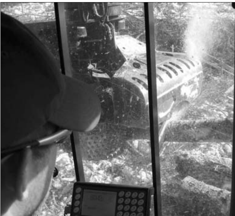
The saw on a tree harvester operated by Douglas Littlejohn cuts through a tree trunk in northern St. Ignace Township. The harvester can cut down a tree, cut off its limbs, and divide the trunk into eight-foot sections in 20 to 40 seconds, depending on the size of the tree.
