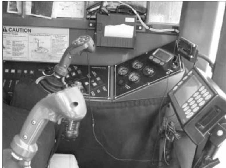
View inside the cockpit of a tree harvester used by Nelson Logging. The operator uses two foot pedals, and two joysticks, with 18 buttons each, to control the movement of the harvester.
