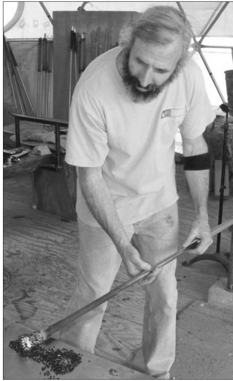
Rick Shapero rolls a glob of clear molten glass on the end of a special tube for blowing glass, along with small pieces of green glass to be made into a goblet. The small green pieces are used to give the goblet a unique swirl design.
